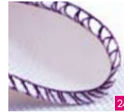
3-thread wrapped overlock narrow Perfect for finishing skirts or as lettuce edge on fine fabrics.
