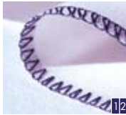
2-thread overlock wide & narrow Finish an edge before you sew fabrics together with a regular straight stitch.
