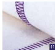
3-thread flatlock, narrow Sew stretchy fabrics together with a decorative effect, either with the flatlock side or the ladder stitch side.
