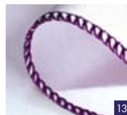
3-thread rolled edge Give a professional finish to silky scarves, pillow ruffles and napkins.
